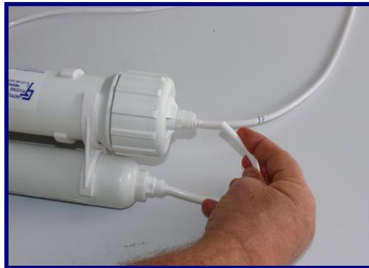
2. **Because the Pre and Post Carbon Filters will release some fines, we have left the line off before the membrane. When installed and ready for use, run water through the first filter until the water runs clear, then push water line into membrane housing firmly.**
